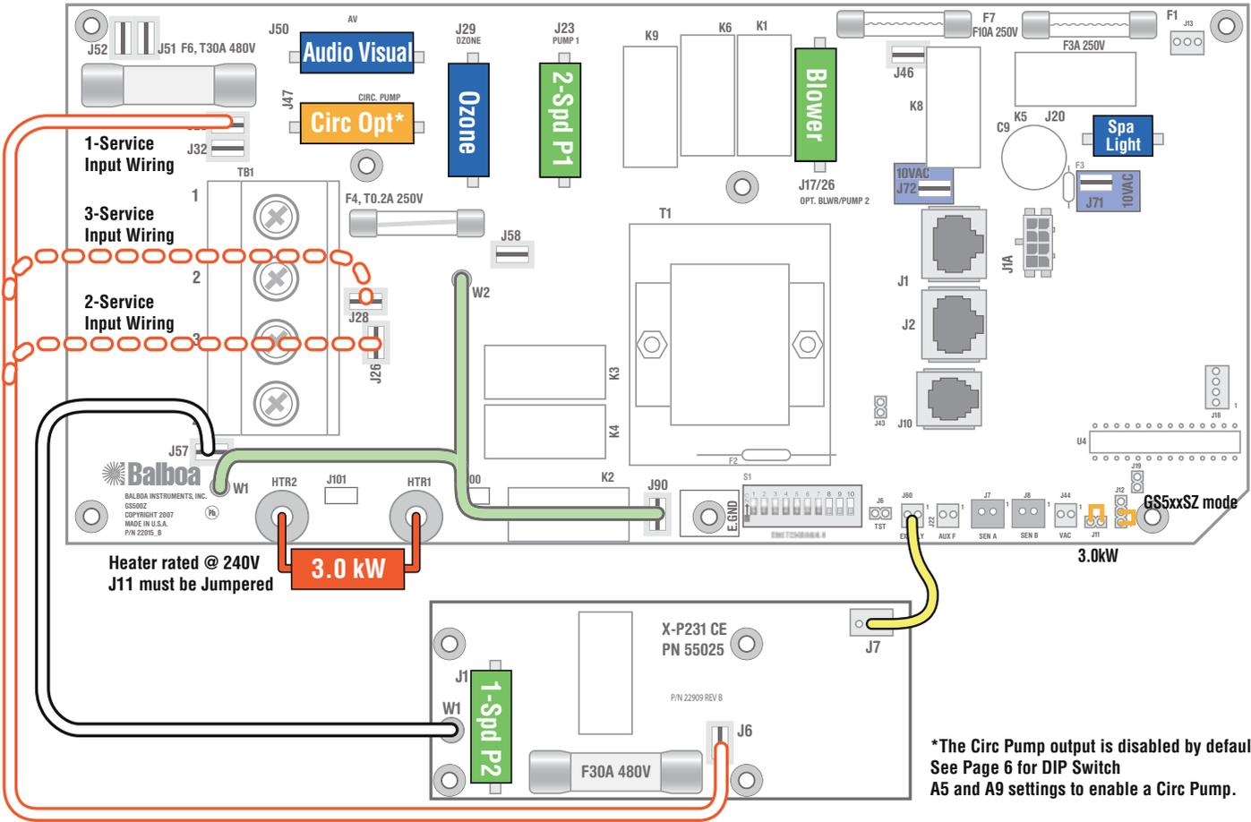
\*The Circ Pump output is disabled by default. See Page 6 for DIP Switch A5 and A9 settings to enable a Circ Pump.
